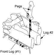
Figure 30 - Installing Crossover Log (#6) (CCL3930PR/NR Shown)
